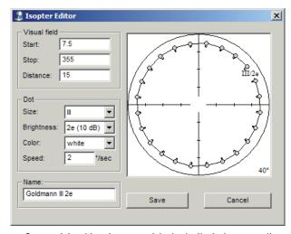
> Customising kinetic tests with the built-in isopter editor
