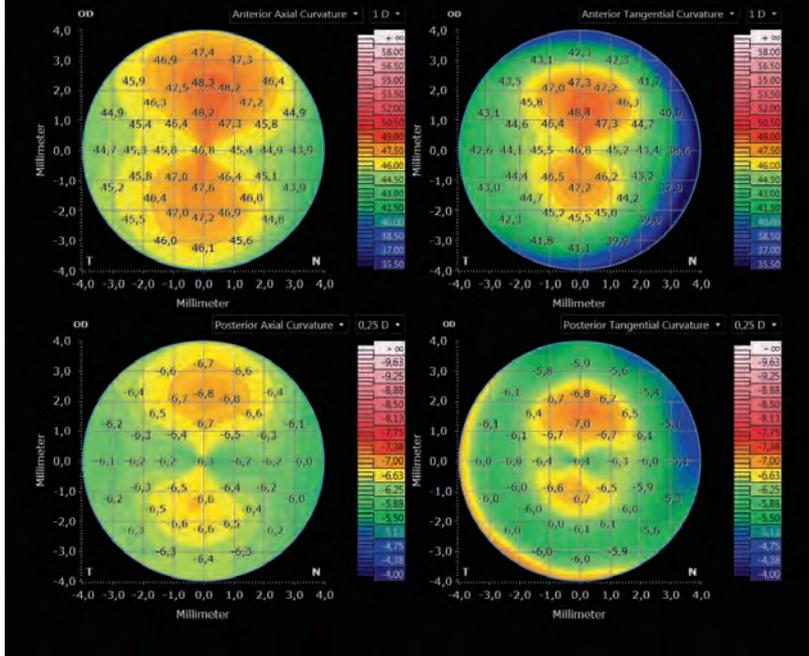
Generate high-resolution images and detailed maps including: camera image, OCT image, anterior and posterior axial curvature maps, tangential maps, elevation maps, total corneal power map, corneal wavefront maps, and pachymetry map.
